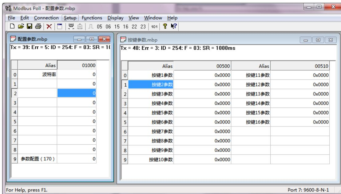
若提示 **Tx = 55: Err = 13: ID = 254: F = 03: SR = 1000ms Timeout Error** 或 **Tx = 55: Err = 10: ID = 254: F = 03: SR = 1000ms Timeout Error**，则表示设备未正常通讯，需检查通讯线和转换器是否正常。
